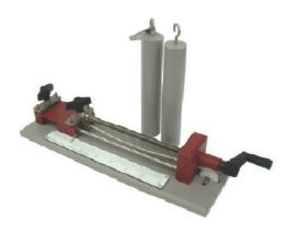
To simply and economically determine the stretch and recovery of textile fabrics, both knitted and woven. The apparatus consists of a loading frame with clamps and a screw tensioning device, two 3 kg loading weights and sample cutting templates.
